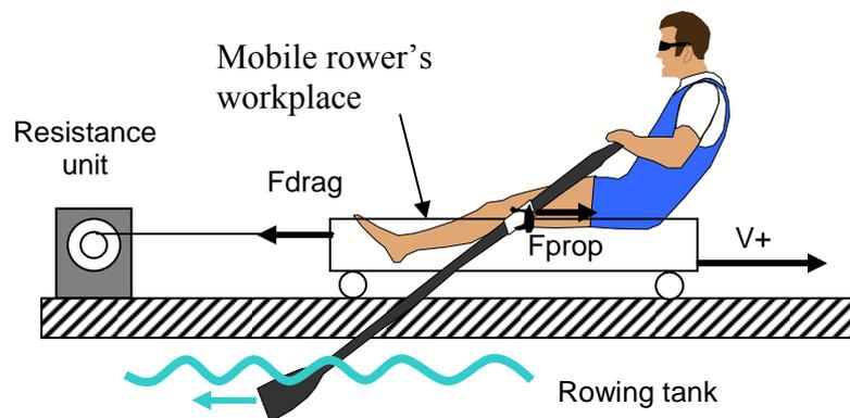
Figure 1. Diagram of the Mobile Rowing Tank
