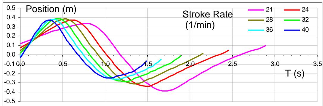
**Figure 2. Position of the carriage during rowing at various stroke rates**
