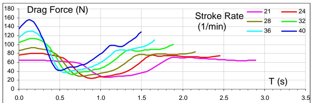
**Figure 3. Drag force applied to the carriage during rowing at various stroke rates**
