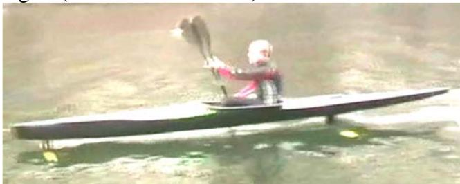
Rowing in a boat with hydrofoils can be used as a speed drill (RBN 2001/4), instead of towing with speed boat. This sort of speed drill can be used more easily, more often and in locations, where speed boats are not allowed (race courses). Ideally, using a hydrofoil would be as easy as using a brake (eg a bungee). Rowers could quickly attach a pair of temporary hydrofoils in the middle of a training session, do their speed work, and then detach them and row normally.
