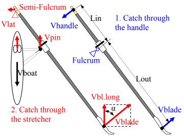
In the first case the blade velocity is equal to:
