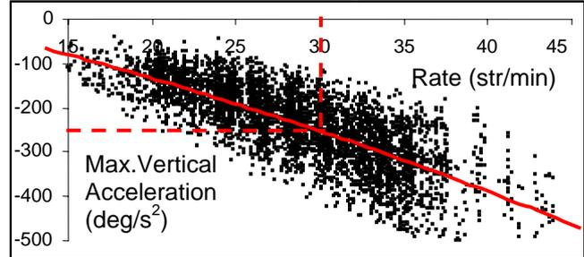
On average, the vertical acceleration exceeds the free fall value at stroke rates higher than 30str/min. This means rowers can “let the blade go” at a low rate, but have to apply upward force at a higher rate. Usually rowers can’t compensate for a higher speed of horizontal movement of the oar at a high rate with a faster vertical movement. Evidence of this fact is the positive correlation of the stroke rate with the catch slip (r=0.24) and release slip (r=0.38).
