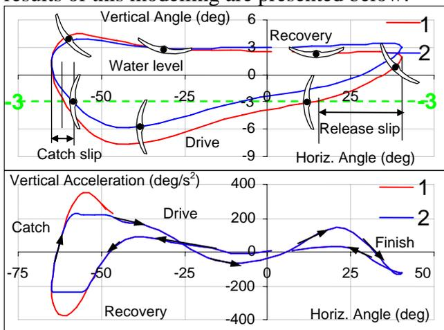
The vertical catch slip was measured from the catch to the point, where the angle of the blade reached -3deg, which corresponds to a fully immersed spoon. You can see that using only free-fall acceleration at the catch nearly doubles the vertical catch slip (from 6.0 deg up to 11.8deg). This increases the slippage of the blade in the water, decreases the blade propulsive efficiency and
