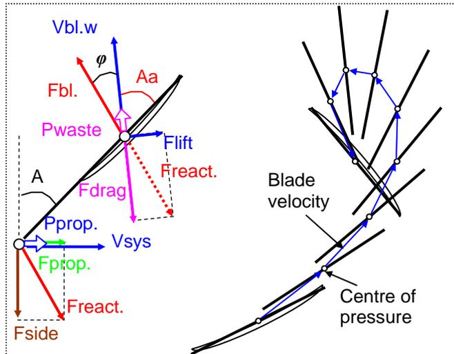
The force applied at the centre of the blade *Fbl* is calculated using measured *Fh* and actual oar gearing (RBN 2006/11). The velocity of the blade relative water *Vbl.w* is determined using oar angular velocity and *Vboat*. The waste power *Pw* is calculated as a scalar product of the force *Fb* and velocity *Vbl.w* vectors:
