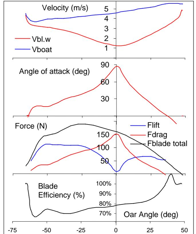
The lift and drag factors were taken from (2) for a flat plate, so they can be used quite approximately here. In this example *Flift* contributes to 56% of the average blade force and *Fdrag* contributes to the remaining 44%. Total distance of the slippage of the blade centre was 1.7m and minimal slippage velocity was 1.25m/s at perpendicular position of the blade. Overall blade efficiency was 76.5%. We will further discuss factors affecting blade propulsive efficiency in future Newsletters.
