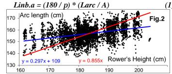
Oar length and span were derived using above gearing ratio leading to more realistic dimensions:
