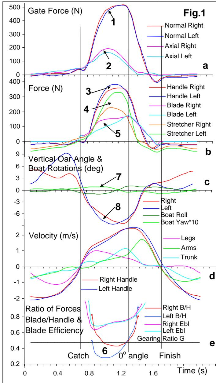
Blade forces  $Fb$  were derived (Fig.1,b) as a difference between normal gate  $Fg$  and handle  $Fh$  forces, neglecting small oar inertia forces:
