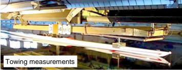
Towing measurements were completely independent from rowing, and all sensors and data processing were provided by the Research Centre. A boat was mounted under a trolley-bridge (56t mass, 4\*200kW engines) running on rails on top of the tank. Each boat was tested at two loads 80kg and 90kg, and at two speeds 4 and 5m/s, with three 500m runs at each load-speed combination – 12 runs for
