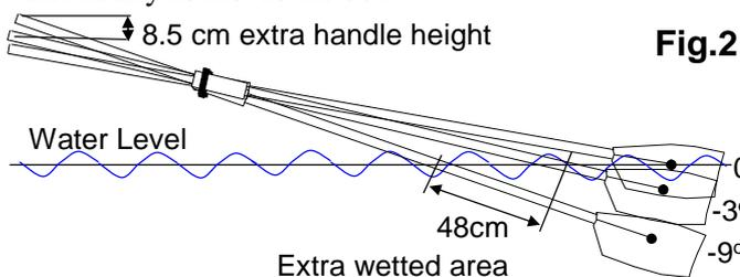
On average, every degree of deeper blade placement put 8cm more of the shaft into the water. So, the difference between normal placement at 6° (40cm of the shaft under the water) and very deep placement at 12° (88cm) is about half a meter extra shaft length in the water (Fig.2). An accurate calculation of the extra drag resistance force  $F_d$  produced
