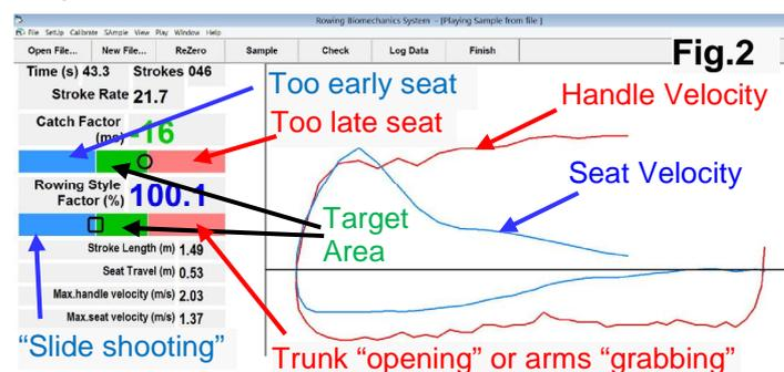
ROWING STYLE FACTOR (RSF) – is the ratio of the seat and handle travels during the first 20% of the drive (about 30cm from the catch). At the most optimal rowing style, this factor should be from 85% to 100%. Numbers
