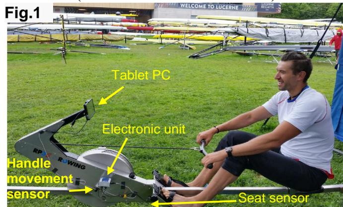
The system is quite simple and consists of a small electronic unit connected to a tablet PC running the BioRow™ software, and only two sensors:
