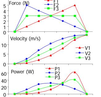
In all cases we have the same total amount of force and power, and the same final speed of the body. However, the front-loaded curve F2 creates the most even power distribution. The back-loaded F1 requires double the peak power. In rowing this late power peak would overload the trunk and arms, which are weaker body segments than legs.
