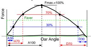
The most obvious parameter is a maximum force Fmax, which is the highest point on the force curve. An average force Faver is equal to the height of a rectangle, of which the area is equal to the area under the force curve. The ratio of the average to maximal forces (Ram=Faver/Fmax) reflects "fat" or "slim" force curves:
