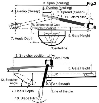
Span (3) in sculling is measured between pin centres at the bottom (because lateral pitch could affect it at the pin top); and spread (3) in rowing is measured from the centreline of the boat to the pin centre. Overlaps (4) could be measured directly, or calculated:
